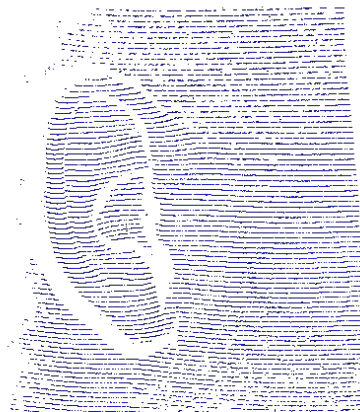
Figure 1: Point cloud data from a single frame of the right ear showing the projected line pattern.
