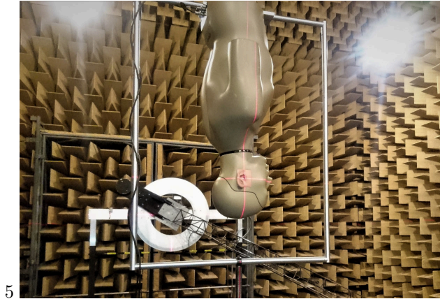
Figure 4: KEMAR in the upside-down mounting rig
